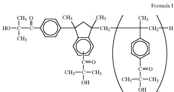
The alpha-hydroxycarbonyl derivatives of oligomers of alpha-methylstyrene are a product with a pour point of from 40 to 50° C. In the present text, this product is indicated as "high viscosity mixture".
