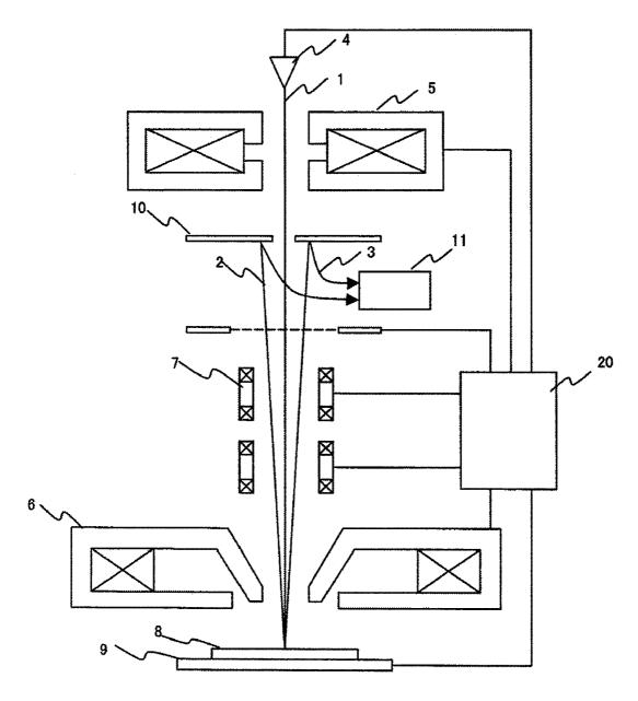
1...PRIMARY ELECTRON BEAM 2,3...SECONDARY ELECTRONS 4...CATHODE
