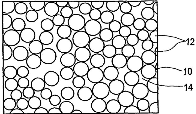
Core wire. Approx. 55 v/o P-25 carbon fiber in Al. matrix 1000 x
