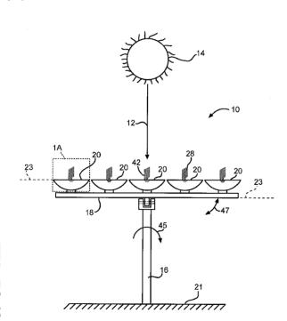
(57) Abstract: In one embodiment, a solar collector includes a heat pipe and at least one cooling fin. The at least one cooling fin is attached to the heat pipe at a non-perpendicular first angle relative to the heat pipe. In further embodiments, methods of transferring heat are disclosed, in addition to methods of manufacturing solar collectors.
