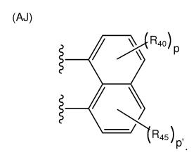
In the structure of Formula (AJ), the variable p is zero or a positive integer from 1 to 3, p' is zero or a positive integer from 1 to 3, and each R<sub>40</sub> and R<sub>45</sub> is independently selected from the group consisting of halogens, alkyl groups, substituted alkyl groups, alkoxy groups, substituted alkoxy groups, aryl groups, and substituted aryl groups.
