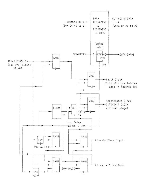
Figure 11: Signal Regeneration Timing
