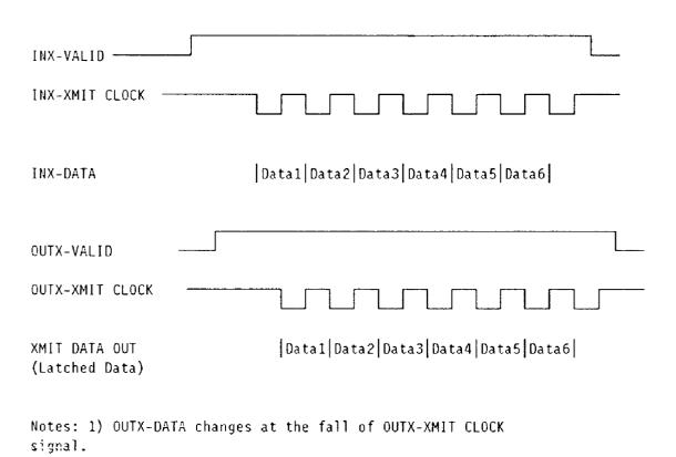
2) INX-DATA is received and latched at the rise of INX-XMIT CLOCK
