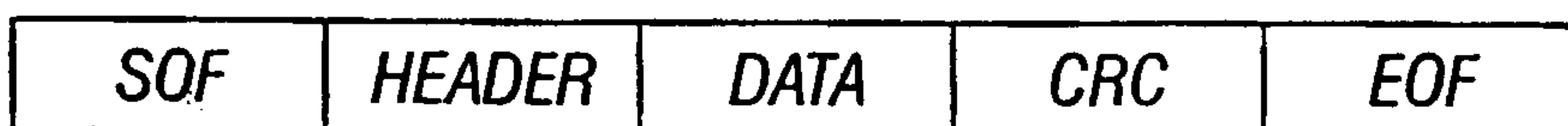
FIBRE CHANNEL FRAME
