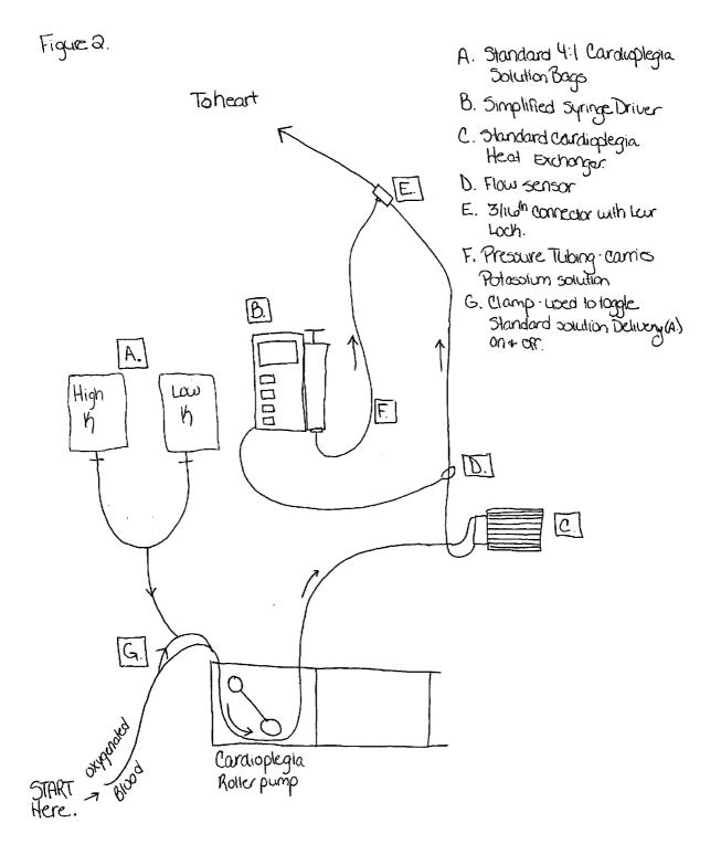
Figure 3. Example Layout of Simplified Syringe Driver.
