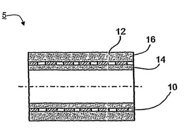
**(57) Abstract:** A medical device comprises a tubular structure adapted for being implanted in the vasculature of a mammal, the tubular structure being formed, at least in part, of electrically charged nonwoven polymer fibers.
