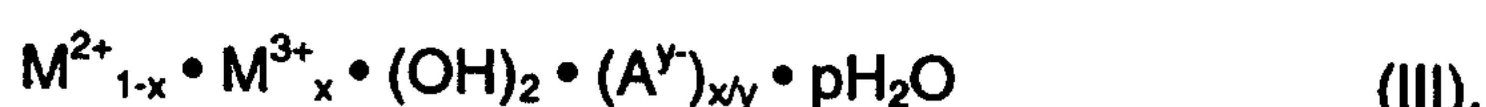
wherein  $M^{2+}$  is Mg or a solid solution of Mg and Zn,  $A^{y-}$  is  $CO_3^{2-}$ , x is a number from 0 to 0.5, and p is a number from 0 to 20.
