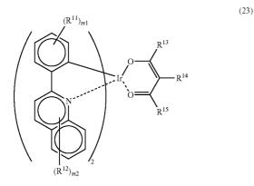
wherein  $R^{11}$  and  $R^{12}$  each represents a substituent;  $R^{13}$ ,  $R^{14}$ and  $R^{15}$  each represents a hydrogen atom or a substituent; m<sup>1</sup> represents an integer of from 0 to 4; and m<sup>2</sup> represents an integer of from 0 to 6.
