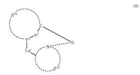
wherein  $Z^{11}$  and  $Z^{12}$  each represent a nonmetallic atom group required to form a 5- or 6-membered ring with carbon atom and/or nitrogen atom, said ring optionally having a substituent or forming a condensed ring with the other ring;  $Ln^1$ represents a divalent group;  $Y^1$  represents a nitrogen atom or carbon atom; and  $b^1$  represents a single bond or double bond. [0016] 4. A compound represented by the following formula (23) or (24) :
