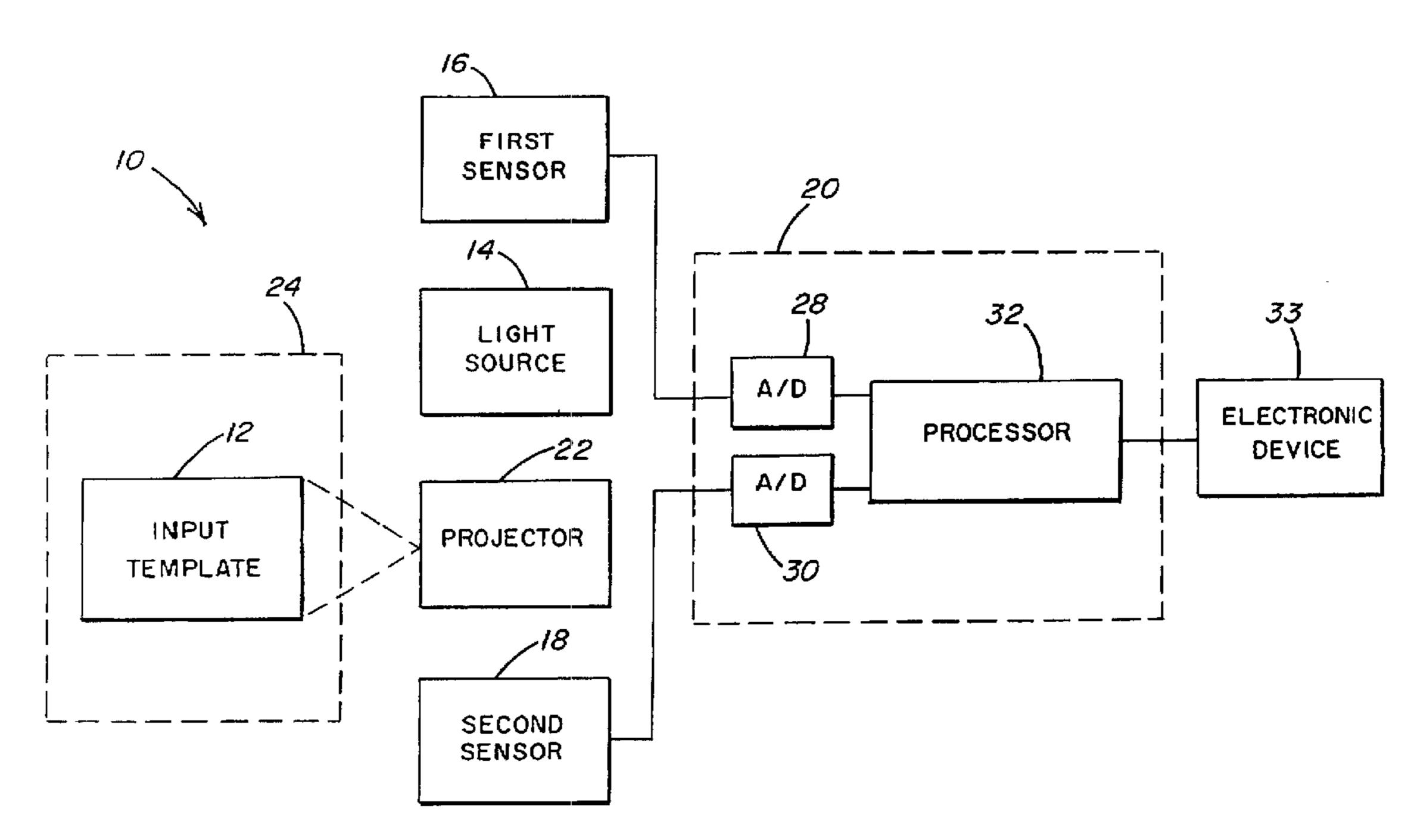
(57) Abstract: An input device (10) for detecting input with respect to a reference plane (24). The input device (10) includes one or more light sensors (16,18) positioned to sense light at an acute angle with respect to the reference plane (24) and for generating a signal indicative of sensed light, and a circuit (20) responsive to said light sensor for determining a position of an object with respect to the reference plane (24).
