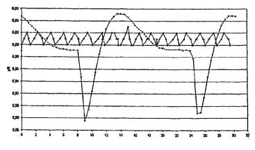
Time [min] -x-pH [1 single stack]; -o-pH [4 parallel REED stacks]
