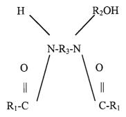
wherein R<sub>1</sub> is an acyclic aliphatic C<sub>15</sub>-C<sub>21</sub> hydrocarbon group and R<sub>2</sub> and R<sub>3</sub> are divalent C<sub>1</sub>-C<sub>3</sub> alkylene groups; commercially available as Mazamide 6 from PPG;
