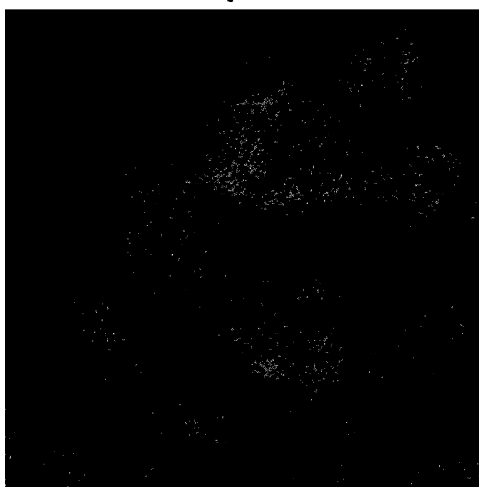
Pd 0.9 -Ru 0.1 alloy fine particles Ru-L EDX map
