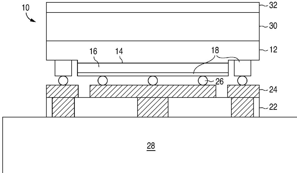
(57) Abstract: Individual side-emitting LEDs are separately positioned in a waveguide, or mounted together on a flexible mount then positioned together in a waveguide. As a result, the gap between each LED and the waveguide can be small, which may improve coupling of light from the LED into the waveguide. Since the LEDs are separately connected to the waveguide, or mounted on a flexible mount, stress to individual LEDs resulting from changes in the shape of the waveguide is reduced.
