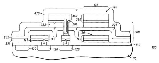
(57) Abstract: A method of manufacturing a semiconductor component includes forming a first capacitor electrode (126) over a substrate (110), forming a capacitor dielectric layer (226) over the first capacitor electrode (126), and forming a second capacitor electrode (326) over the capacitor dielectric layer (226). The capacitor dielectric layer (226) is made of aluminum.
