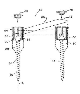
(57) Abstract: A minimally invasive method for stabilizing adjacent vertebrae to be fused is accomplished with a device configured to interlink the pedicles of the adjacent vertebrae and. including multiple pedicle screws (54). Each of the pedicle screws (54) has a screw head (60) configured to receive a connecting rod (66) in a position, in which the rod (66) and the receiving pedicle screw (54) are vertically aligned.
