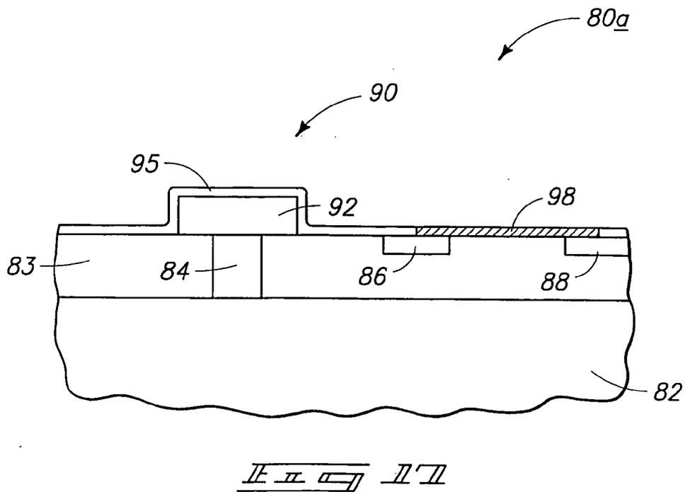
**METHODS OF FORMING CONDUCTIVE CONTACTS TO SOURCE/DRAIN REGIONS AND METHODS OF FORMING LOCAL INTERCONNECTS**
