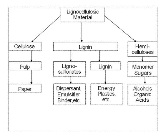
Figure 1 Products from fractionation of lignocellulosic material in alcohol, water and sulfur dioxide.
