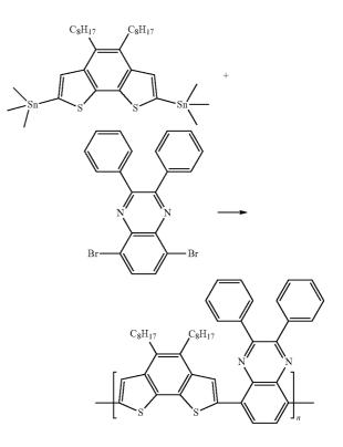
**[0057]** The detailed preparation procedure is: under the protection of nitrogen, a solution of compounds 5,8-dibromo-2,3-bis(phenyl)quinoxaline (0.22 g, 0.5 mmol) and 2,7-bis-trimethyltin-4,5-dioctyl-benzo[2,1-b: 3,4-b']dithiophene (0.37 g, 0.5 mmol) in chlorobenzene (20 mL) was bubbled with nitrogen for 0.5 h to remove the oxygen in the environ-
