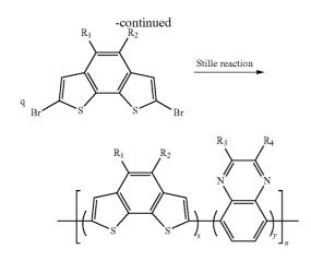
**[0039]** Compounds A and C in the above step (1) may be prepared according to the step (2) of Example 1, and the method for producing compound B preferably includes following steps:
