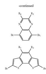
**[0035]** wherein,  $R_1$  and  $R_2$  are independently selected from  $C_1 \sim C_{20}$  alkyl,  $R_3$  and  $R_4$  are independently selected from the group consisting of —H,  $C_1 \sim C_{20}$  alkyl,  $C_1 \sim C_{20}$  alkoxyl, benzene ring group containing alkyl or alkoxyl, fluorenyl group containing alkyl and carbazyl group containing alkyl;
