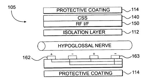
(57) Abstract: Provided is an implantable RFID-enabled micro-electronic neurostimulator system comprising (a) an internal subsystem having (i) an array of electrodes, where at least one electrode pair contacts a nerve; (ii) a multiplexer; (iii) digital to analog signal converter; and (iv) a RFID based control and stimulation chip; and (b) an external subsystem having (i) a controller; and (ii) an RP interface.
