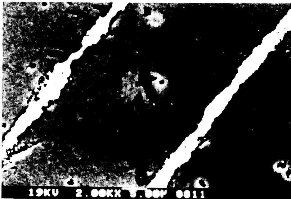
Fig 1. A multilayer capacitor with stable temperature characteristics containing Nb_2O_5 in the dielectric composition.
