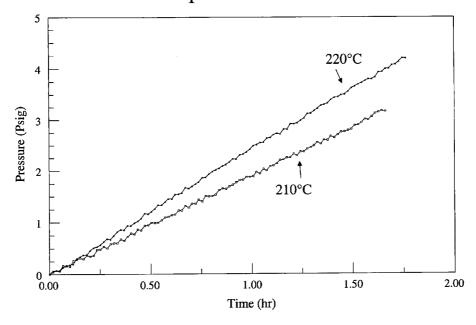
Hydrogen Production Using Carbon And Solid NaOH FIG-At Different Temperatures In 40 mL Container 220°C 1.50 210°C Time (hr) 0.50 Pressure (Psig)
