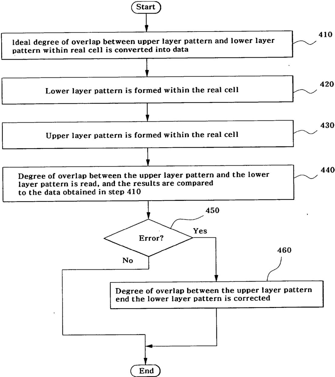
**OVERLAY VERNIER AND METHOD FOR MANUFACTURING SEMICONDUCTOR DEVICE USING THE SAME**
