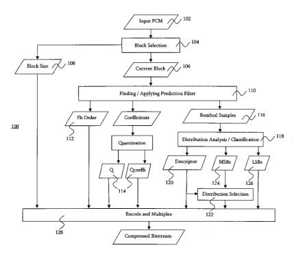
(57) Abstract: Compression of audio signal data is described herein. In various embodiments, the compression of each unit of the audio signal data includes the employment of a distribution substantially representative of a subblock of residual data of the unit of audio signal data, to reduce the amount of data having to be transmitted to transmit the unit of audio signal data to a recipient.
