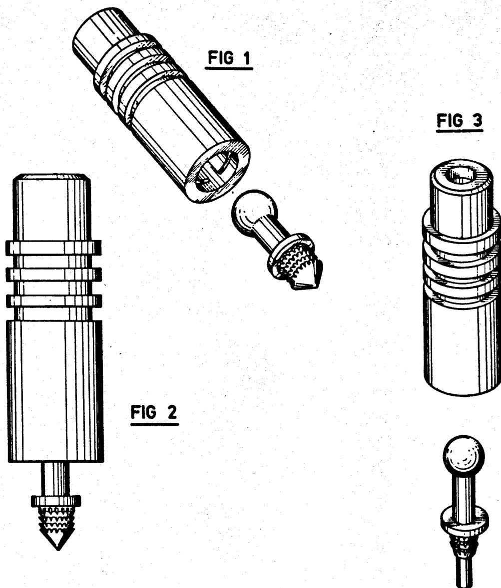
FIG. 1 is an exploded view of an electrical connector according to my design;
