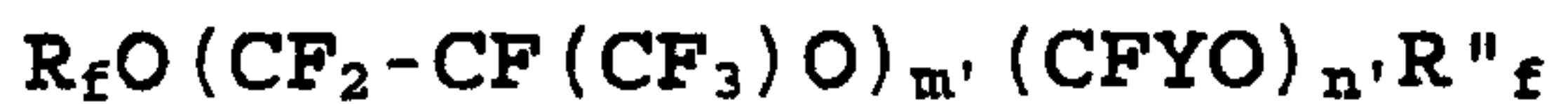
having a random distribution of the perfluoroxyalkylenic units, wherein  $R_f$  and  $R''_f$  equal to or different from each other are neutral end groups as defined above,  $m'$  and  $n'$  are integers selected to meet the above requirements of molecular weight, Y has the meaning indicated above; the surfactant based on perfluoropolyether has the following formula:
