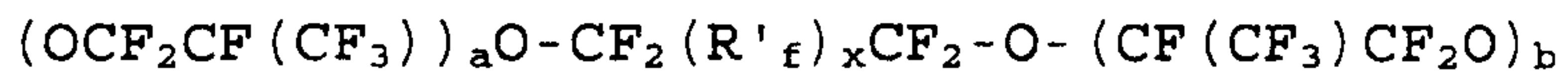
wherein  $R'_{\text{f}}$  has the meaning indicated above, x is 0 or 1, a and b are integers and a+b is at least 1 and such that the molecular weight is that indicated above;
