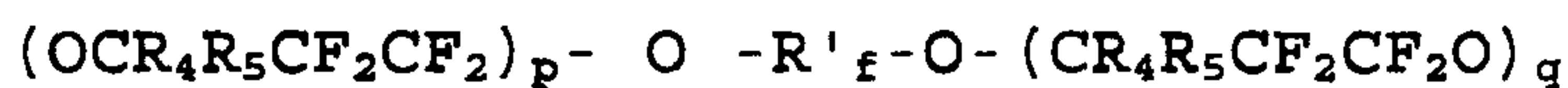
wherein  $R'_{\text{f}}$  is a fluoroalkylenic group, p and q are integers from 0 to 200, and p+q is at least 1 and such that the molecular weight is that indicated above;
