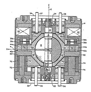
ther network detects rotational displacement of the rotor about the input axes and generates appropriate signals for torquers (72, 76) which serve to maintain the rotor in a position where its spin axis is substantially coincident with the spin reference axis.
