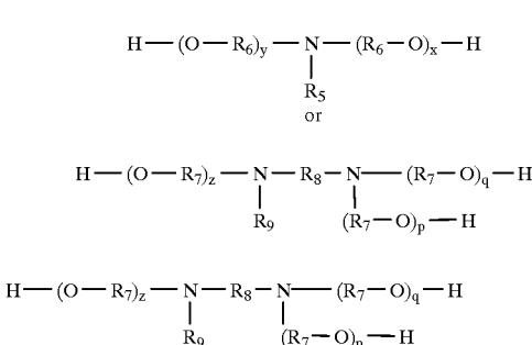
wherein  $\text{R}_5$  and  $\text{R}_9$  are independently  $\text{C}_1$  to  $\text{C}_{30}$  hydrocarbyl radicals,  $\text{R}_6$  and  $\text{R}_7$  are independently  $\text{C}_2$  to  $\text{C}_6$  hydrocarbyl radicals,  $\text{R}_8$  is a  $\text{C}_1$  to  $\text{C}_6$  hydrocarbyl radical,  $x$  and  $y$  are integers from 0 to 50 provided that  $0 < (x+y) \leq 50$ , and  $p$ ,  $q$  and  $z$  are integers from 0 to 50 provided  $0 < (p+q+z) \leq 50$ .
