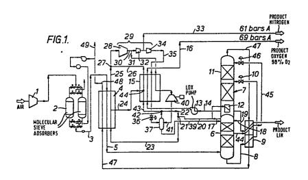
This invention relates to a method for producing gaseous oxygen and to a cryogenic plant in which said method can be carried out.
