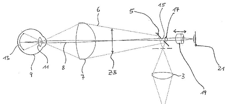
(57) Abstract: The invention relates to a device for observing the ocular fundus, in particular to a fundus camera. Said device comprises a light source (1b) for the provision of illumination radiation, an illumination optical path for directing the illumination radiation onto the ocular fundus and observation optics for reproducing the illuminated ocular fundus, the observation optics comprising a module (16b), whose refractive power can be electrically adjusted.
