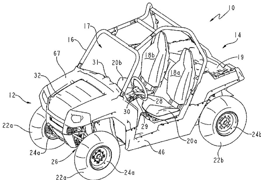
(57) **Abstract:** The present invention relates to all terrain vehicles (10) having at least a pair of laterally spaced apart seating surfaces (18a, 18b and 20a, 20b). More particularly, the present invention relates to trail compliant side-by-side all terrain vehicles (10).
