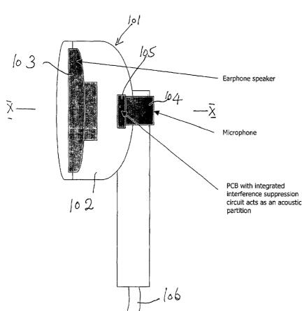
(57) Abstract: In or for use with a portable communications device, a device which comprises an earpiece having a loudspeaker and a microphone mounted thereon. An apparatus for use with a portable communication device, said apparatus having a compartment therein which accommodates a flex which connects said portable communications device to an earpiece.
