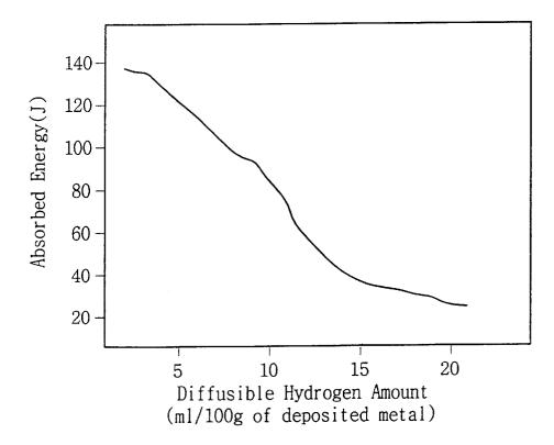
METAL CORED WIRE FOR GAS SHIELDED ARC WELDING HAVING EXCELLENT ZINC PRIMER RESISTANT PERFORMANCE AND LOW TEMPERATURE IMPACT TOUGHNESS
