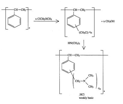
The disadvantage of this process is an unavoidable <sup>55</sup> secondary reaction in which the basic nitrogen reacts with more than one halogen radical. This results in crosslinking to form quaternary structures having undesired strongly-basic ion exchanger properties (R. L. Gustarson, Ind. Eng. <sup>60</sup> Chem. Fundam., Vol. 9, No. 2, 1970), the exchange capacities being reduced.
