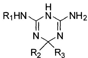
The synthesis involves the reaction of a mono-substituted bisguanidine and an aldehyde or ketone in presence of an acid at elevated temperatures.
