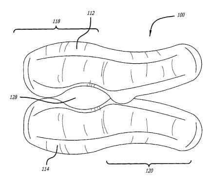
(57) Abstract: A child-safe fastening device comprises a clip, one or more than one padded layer covering one or more surfaces of the clip, and one or more than one cover layer secured to the padded layer. The clip, the padded layer, and the cover layer form a plush device.
