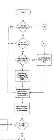
(57) Abstract: A shooting system provided by using a firearm having a telecospic gun sight (10) mounted a predetermined distance above the barrel in conjunction with a computer (figure 18 a-g) including a controller, memory; a program stored in memory for calculating targeting information (figure 16a).
