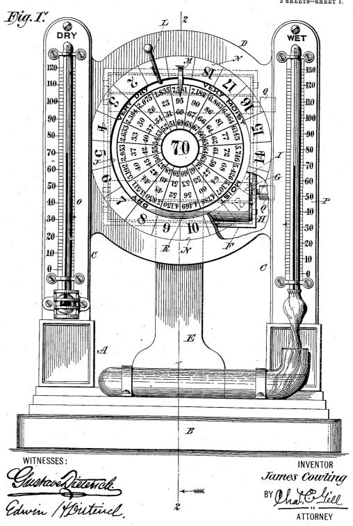
J. COWLING. HYGROMETER. APPLICATION FILED JULY 21, 1906.
