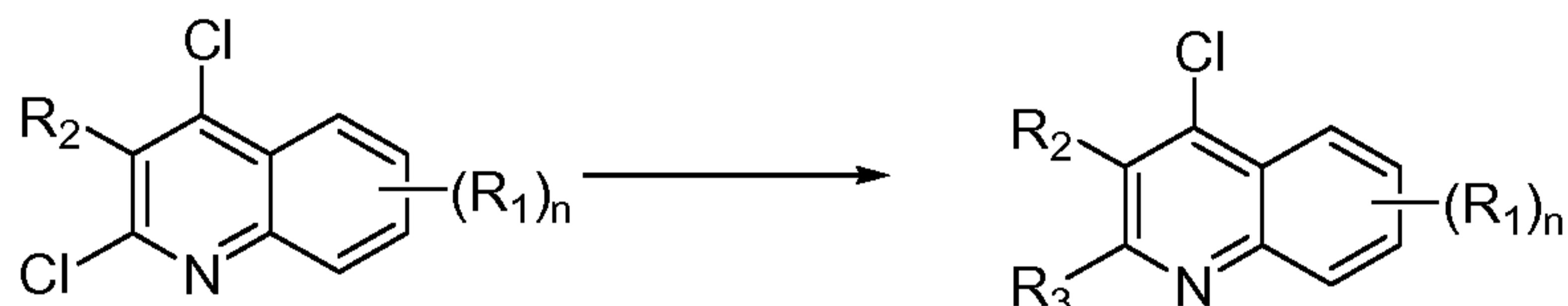
5 A mixture of the substituted dichloroquinoline (1 equiv.), the boronic acid (1 equiv.), sodium carbonate (2 equiv.) and tetrakis(triphenylphosphine)palladium (0.1 equiv.) in toluene-water (5:2, 0.15M) was heated at reflux overnight. After this time the reaction was cooled to rt and treated with EtOAc and water. The separated organic layer was dried over magnesium sulfate, filtered and evaporated 10 *in vacuo*. Column chromatography gave the substituted 4-chloro quinolines.
