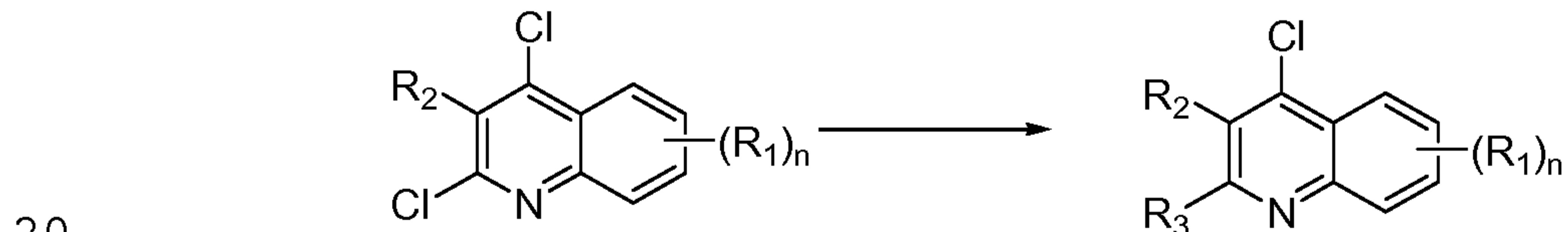
20 A mixture of the substituted dichloroquinoline (1 equiv.), the Stille reagent (1 equiv.) and tetrakis(triphenylphosphine)palladium (0.1 equiv.) in toluene (0.21M) was heated at reflux overnight. After this time the reaction was cooled to rt and treated with EtOAc and water. The separated organic layer was dried over
