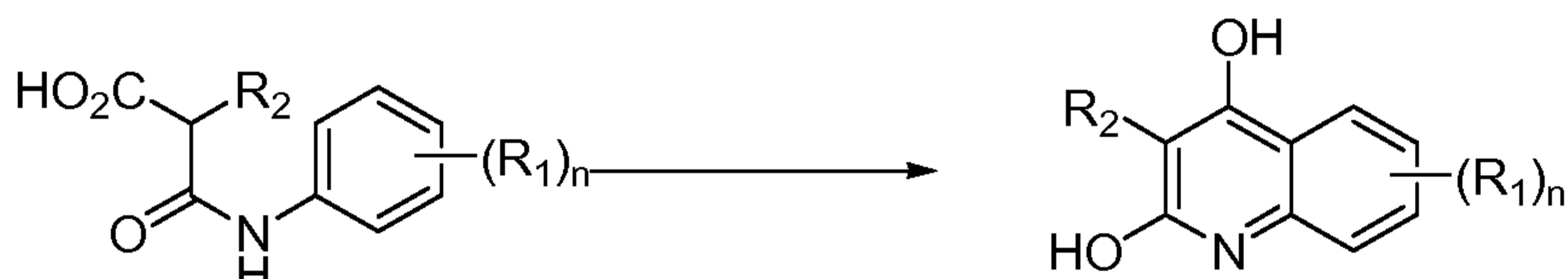
5 A mixture of phenylamino-oxopropanoic acid in polyphosphoric acid (0.6M) was stirred at 130 °C for 2 h. After this time the reaction was cooled to rt and treated with 2M aq. sodium hydroxide until a precipitate formed. The precipitate was filtered and washed with 1M aq. sodium hydroxide and dried under vacuum to give substituted quinoline diols.
