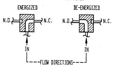
N.D.=NDRMALLY OPEN VALVE PORT (CLOSES WHEN VALVE IS ACTUATED)
