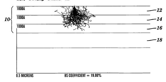
MONTE-CARLO SIMULATION OF 5KeV BALLISTIC ELECTRON INJECTION INTO A COMPOSITE INSULATOR
