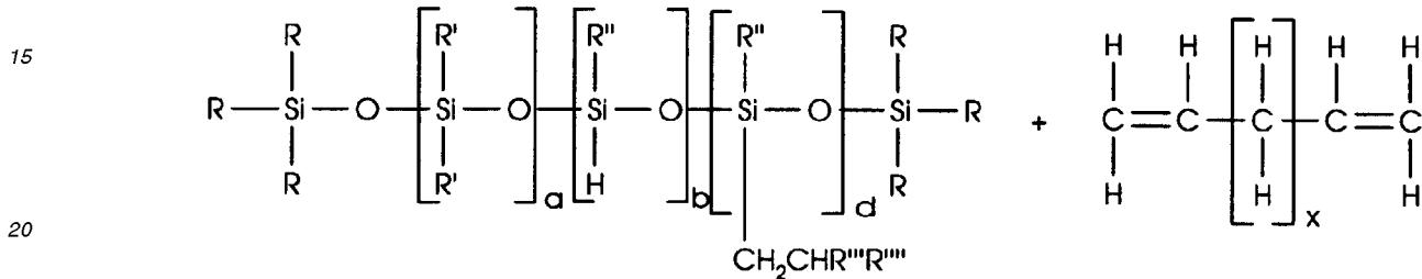
**Fluid/Solvent + Pt Catalyst → G + Fluid/Solvent + Shear → Paste**
