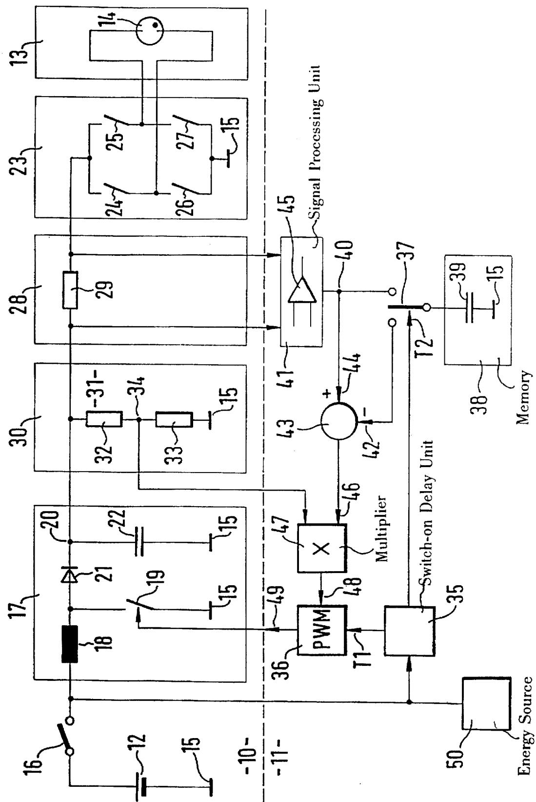
**CIRCUIT ARRANGEMENT FOR PROVIDING SIGNAL CORRECTION INCLUDING A SWITCH-ON DELAY TIME PERIOD DURING WHICH A CORRECTION SIGNAL IS DETERMINED FOR USE DURING A FOLLOWING TIME PERIOD**
