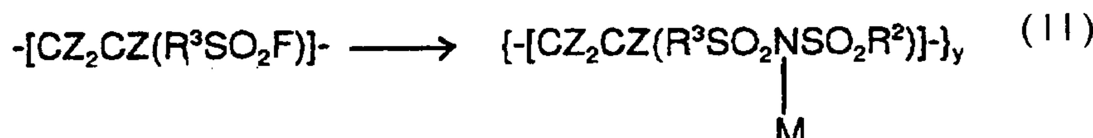
(57) Abstract: This invention discloses a method for preparing imides (I) and (II) from compounds having a sulfonyl fluoride functional group. The imides so prepared are useful in a variety of catalytic and electrochemical applications. (I) or polymer comprising the unit (II)
