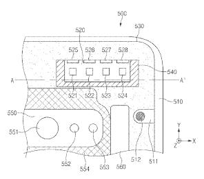
between the antenna module and the injection-molding material when viewed from the second plate in a direction of the first plate. A partial conductive radiator of the conductive radiators may be disposed to transmit and/or receive a signal through the second plate.
