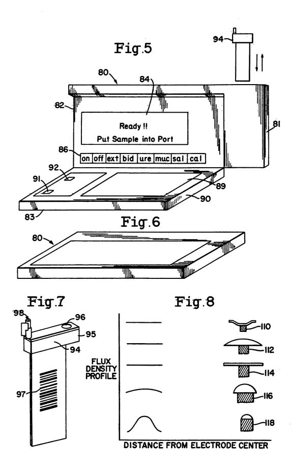
UNIVERSAL SENSOR CARTRIDGE FOR USE WITH A UNIVERSAL ANALYZER FOR SENSING COMPONENTS IN A MULTICOMPONENT FLUID
