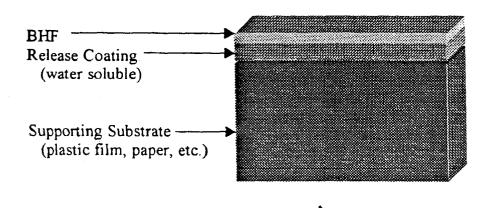
Moisten the backside of the composite device with water and the transparent BHF film will release as a free film as shown below.
