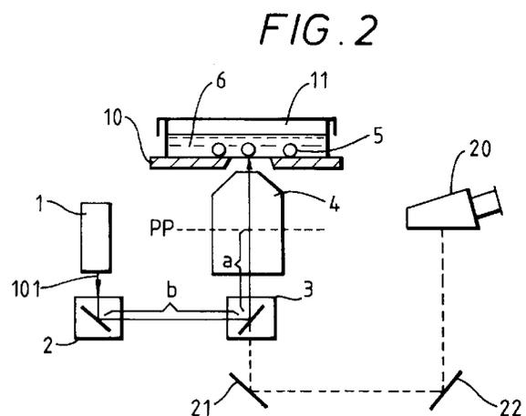
This invention relates to apparatus and methods for applying a laser beam through a microscope, in particular an inverted microscope.
